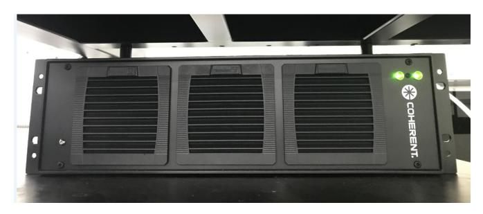
The power on without fault as green indicator . The DC 48V power supply output 48V to laser head normally .
